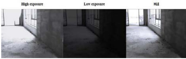
Figure 4. High and low exposure frames captured by the Intel Realsense 435 camera and processed frame in the HLE method.
